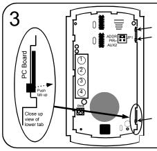
Remove the PC Board by bending back 3 tabs holding the PC board in place. Pull board up slightly and away from opposite side of FTPBR Touchpad housing to remove.
