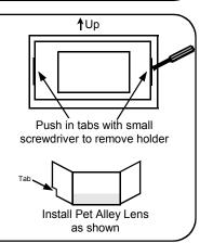
**5** Secure lens by snapping the PIR lens holder back into place. Be sure both tabs are securely fastened to the F-TPBR Touchpad housing. **Note:** Be sure grooved side of lens is facing in (smooth side is facing out).
