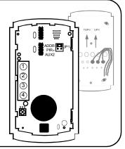
2 In the center of the PC board is a speaker, with black and red wires connected to a plug mated to a receptacle. Remove the speaker plug by pushing back the retainer latch on the receptacle using a small screwdriver and carefully pulling plug out of the receptacle.
