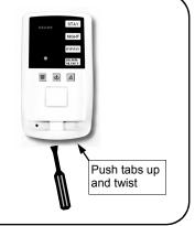
Mark the holes. Mount anywhere in a room with a favorable PIR field of view, approximately 60" high (measured from the floor to the top of the FTPBR Touchpad).
